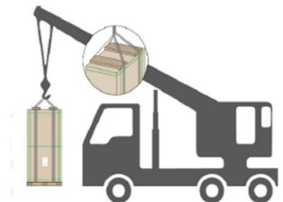
Before hoisting, check whether the pallets and cartons are damaged and whether the hoisting ropes are strong and firm. When the lifting is about to hit the ground, one person on each two side should upright the carton gently on the relatively flat position of the project ground.
