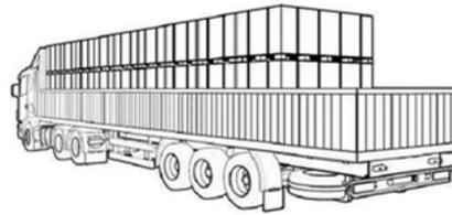
Packaged products can be shipped by land, sea, or air. During transportation, please fix the packing box on the transport platform to ensure that the packing will not roll over (Take land transportation as an example).
